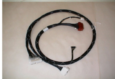
Power Distribution Harnesses
